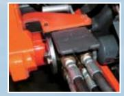
Single-lever Hydraulic Quick Coupler The optional quick coupler allows the operator to attach all four hoses at once. This makes attaching and detaching fast and easy, even when you're doing it often.
