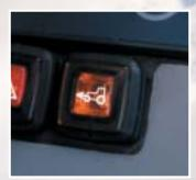
Hydraulic 4WD Engagement With the press of a button, 4-wheel drive can be activated and deactivated without stopping the tractor.
