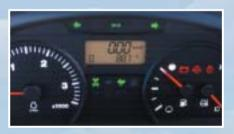
The new instrument panel makes viewing the vital functions of the tractor clear and easy. The LCD readout displays travel speed, PTO revolution and hour meter information digitally. Illuminated analog indicators include a large tachometer, temperature gauge and fuel gauge.
